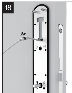
The Outside Trim data cable connects to rear panel data cable, please tuck in the door if the cable is too long
