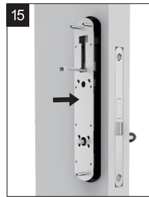
The rear back plate is mounted on a silicone pad
