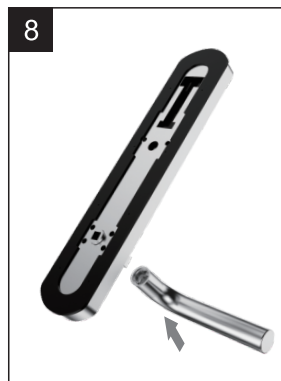
Press the module and change the handle direction
