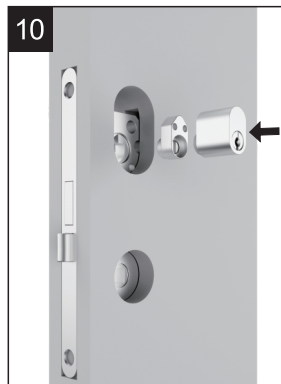
Press the module and change the handle direction
