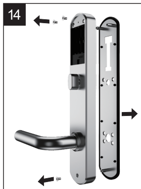
Installation the Outside Trim like this
