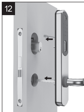
Installation the Outside Trim like this
