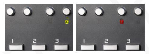
If a reading not is indicated, the credential lacks compatibility, or that the MIFARE or EM reading has been disabled. This is set in the in the VAKA software under *Settings*, *Card/Code*, *Cards*.
